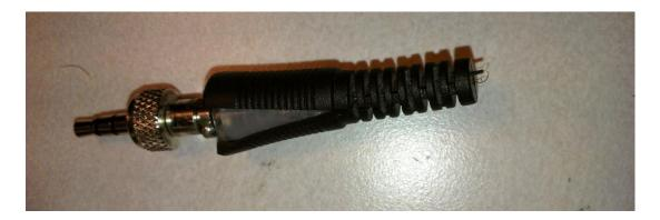
3. Pull the connector and wire out of the strain relief
