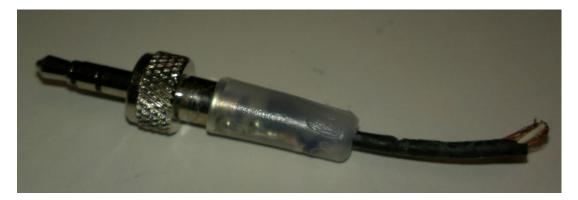
4. Cut through the white cable mold on both sides
