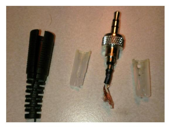
5. Notice the small piece of shrink tube the isolates the 2 wires
